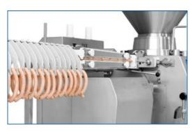
The RHS 230 by REX is the effective solution to hang the sausages immediately after twisting-off, It is connected either to the RKS 85 or directly to the casing holder of the vacuum filler. From there, the twisted-off sausage chain is taken up immediately by the hooks of the RHS and hung, to allow their removal with the smoke bar.
