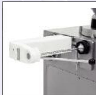
casing holding device, fixed for natural casings
